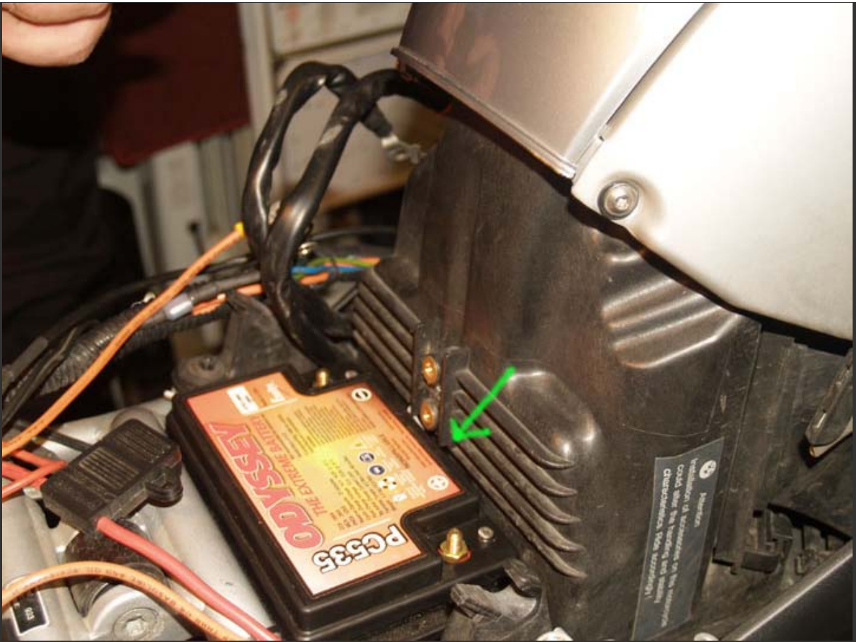
Place the battery in the box and check clearances. The ridge, arrow, will need about 1/8" trimmed off.
